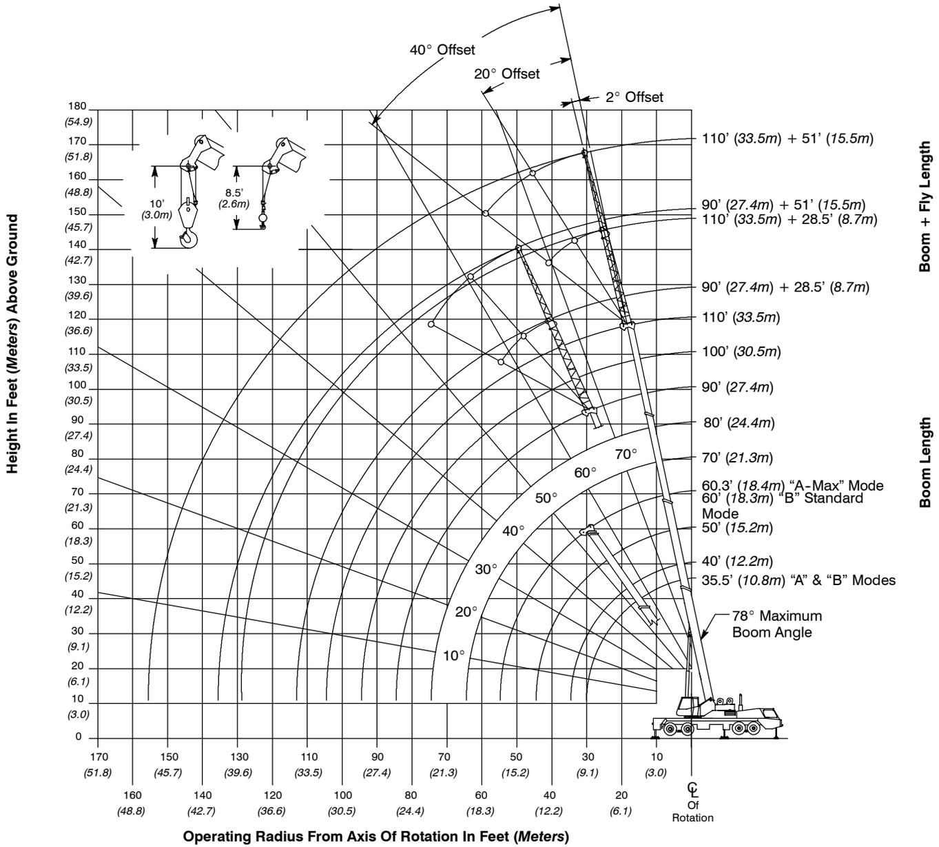
**Note: Boom and fly geometry shown are for unloaded condition and crane standing level on firm supporting surface. Boom deflection, subsequent radius, and boom angle change must be accounted for when applying load to hook.**
